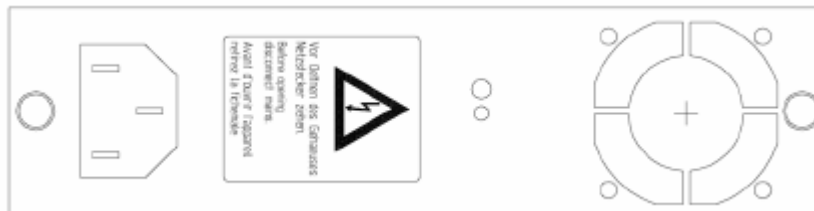
Figure 4: 100 ... 240 VAC power supply and fan modules
